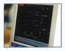
The ventilator has ergonomic layout for easy handling. The vital patient data with the alarm thresholds are placed in vertical column on the right of the panel. The data include monitored FiO<sub>2</sub>, Plateau Pressure, inspired and expired Tidal Volume.
